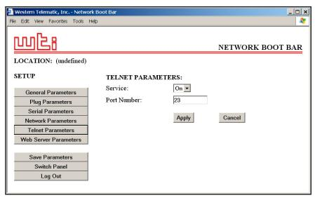
Figure 5.12: Telnet Parameters Menu - Web Browser Interface
